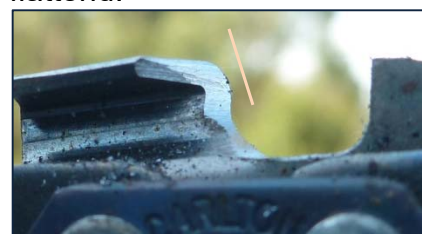
File too large, cutting edge flattend.
